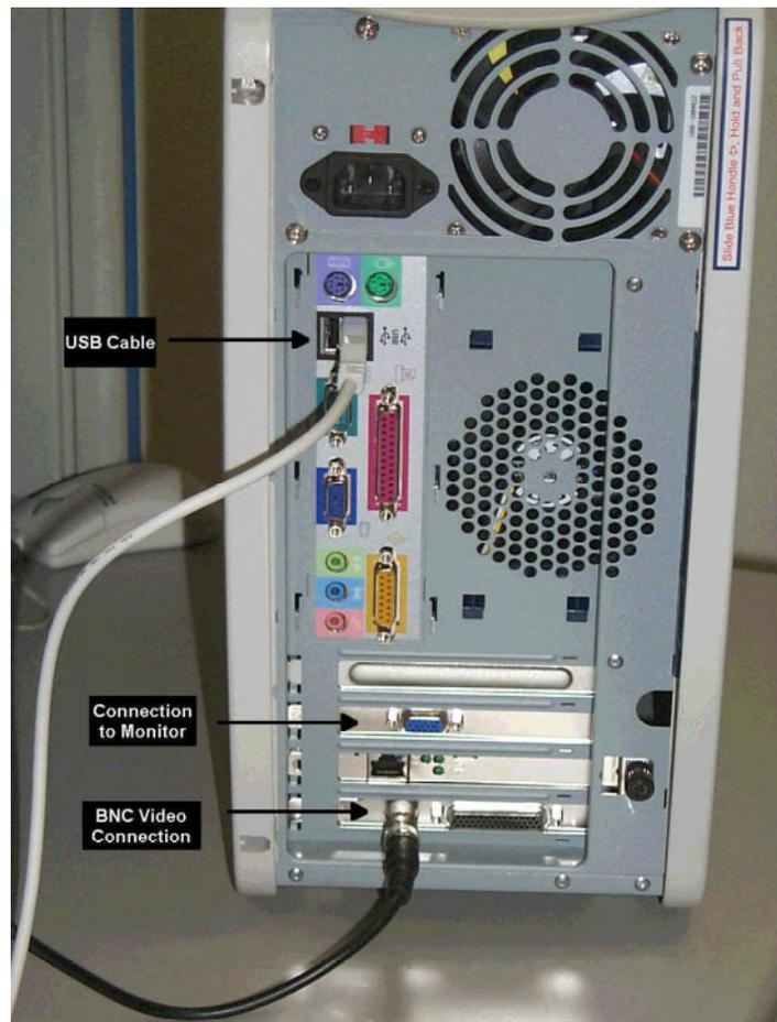
**Figure 4. USB Connections.**
