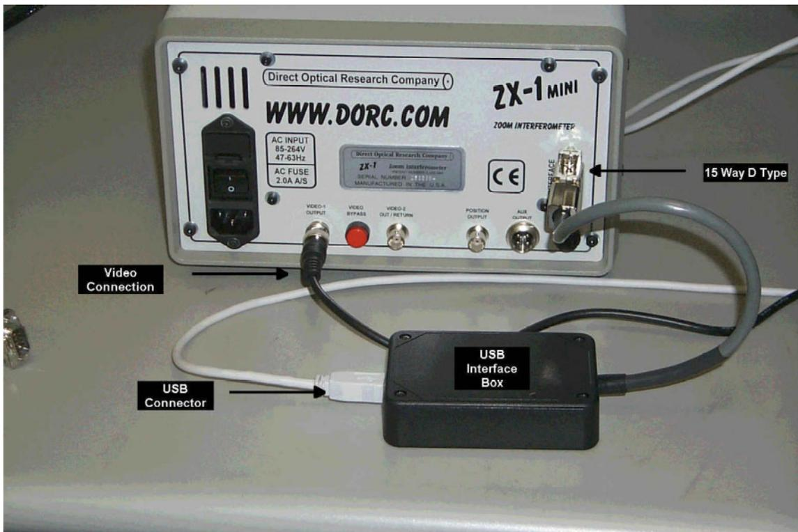
**Figure 5. ZX-1 Mini PMS and USB Interface Box Connections.**
