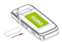
• Then close the MicroSD card slot cover. The driver of the MicroSD card will installed automatically when the modem driver is installed.
