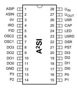
Figure 2: Pin Configuration, 28-Pin SSOP
