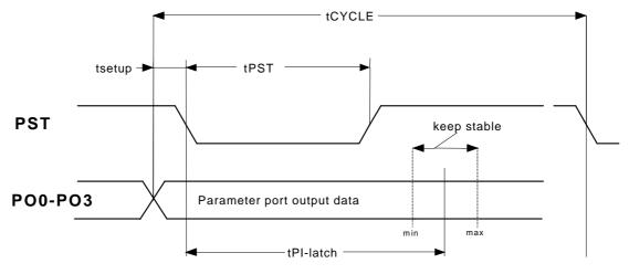
parameter input value (PIx) = parameter output value (POx) wired AND with external signal source value
