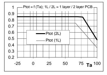
Figure 6: Maximum Power Dissipation,  $P_{TOT} = f(Ambient Temperature)$
