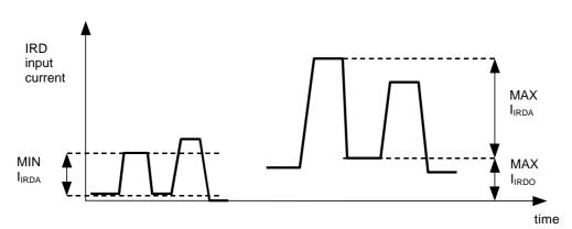
Figure 10: Photo Current Waveform
