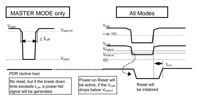
Figure 12: Power-Fail Generation (in Master Mode) and Reset Behavior (All Modes)
