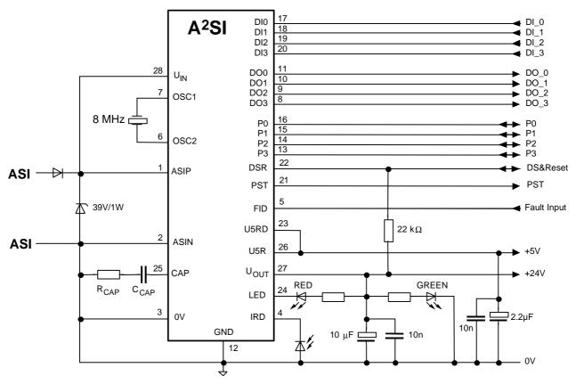
Figure 13: Typical Application, Slave Mode
