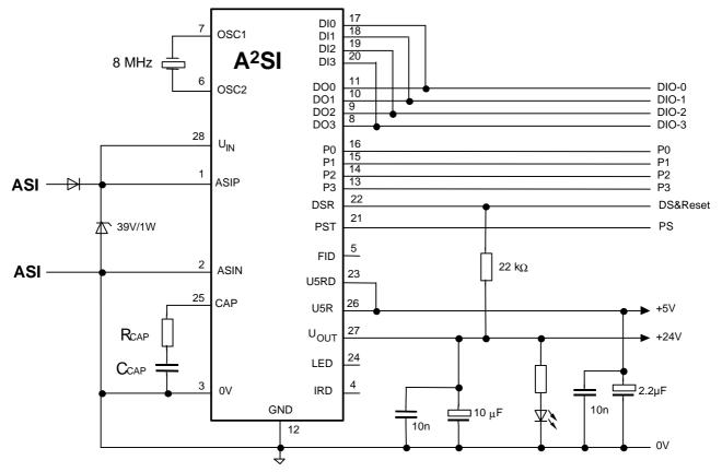
Figure 14: Typical ASI3+ Compatible Application
