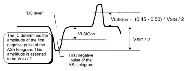
Figure 11: Receiver Comparator Set Up
