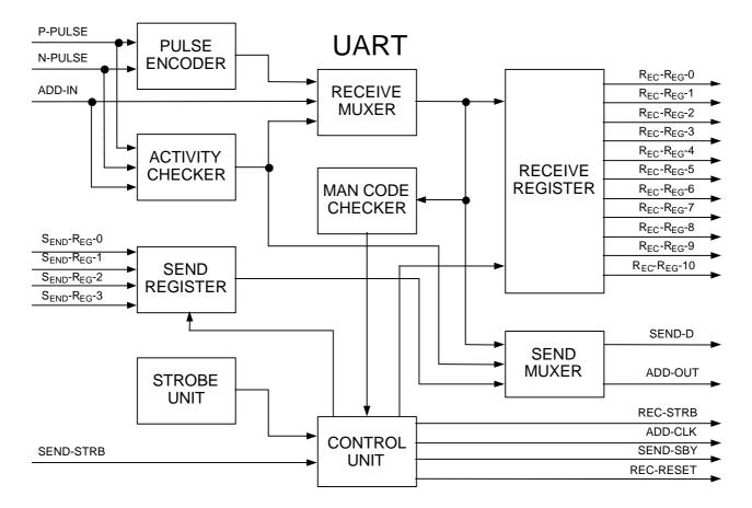
Figure 5: UART Block Diagram
