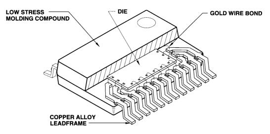
Figure 16: SSOP Package
