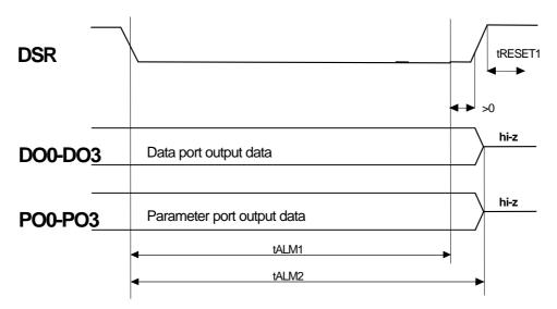
Figure 9: Timing Diagram External Reset via DSR
