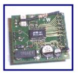
Figure 19: Evaluation board dimensions (L x W x H):(34 x 31 x 8) mm<sup>3</sup>
