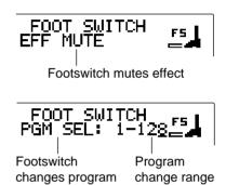
Use the REV TIME control to switch between the EFF MUTE and PGM SEL functions. If you select the former, the REV500's effect output will be suppressed when you depress the footswitch. Depress the footswitch again to release the effect mute.
