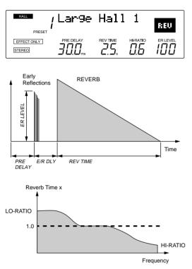
The four PARAMETER EDIT controls on the REV500's front panel let you adjust the basic program parameters quickly and easily. When you rotate one of these controls, the program information in the LCD (shown above) will be replaced by a graphic display indicating how the changes you've made have affected the parameter in question. (The display will return to normal a few moments after you stop turning the control.)
