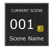
The Scene Memory area in the Mixer window also functions as a button which can be pressed to access the Scene Memory window.
