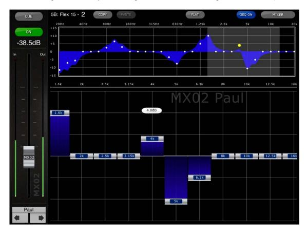
The current channel's Name, Fader, Level Meters, [ON] and [CUE] buttons are shown in the left column. At the bottom-left, there are "previous" and "next" arrow buttons for navigating to different channels. Pressing these buttons will only access other channels that have GEQs assigned to them.
