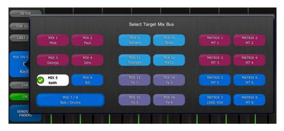
Choose from Mix 1-16 and Matrix 1-8. The currently selected Mix will appear as a white button with a check mark. Stereo pairs appear as single large buttons.
