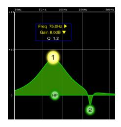
In some cases, it may be necessary to adjust the gain without altering the frequency. Or to adjust the frequency without changing the gain. In this case, the "Gain Lock" or "Frequency Lock" functions can be used. These buttons are located at the top of the EQ graph.
