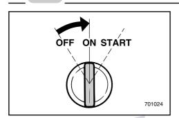
2) Turn on the main switch. The oil injection system will automatically feed oil from the remote oil tank to the engine oil tank.
