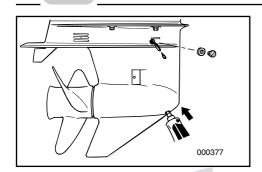
5) With the outboard motor in a vertical position, and using a flexible or pressurized filling device, inject the gear oil into the oil drain plug hole.
