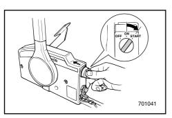
8) Press in and hold the main switch to operate the remote choke system.(The remote choke switch returns to its home position when you release your hand. Therefore, keep the switch pressed in.)
