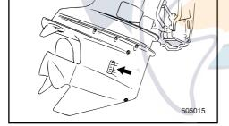
If the warning system has been activated, stop the engine and check the water inlet for clogging.
