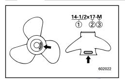
Yamaha outboard motors are fitted with propellers chosen to perform well over a range of applications, but there may be uses where a propeller with a different pitch would be more appropriate. For a greater operating load, a smaller-pitch propeller is more suitable as it enables the correct engine speed to be maintained. Conversely, a larger-pitch propeller is more suitable for a smaller operating load.
