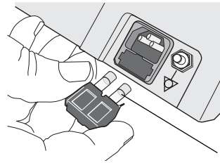
Figure 57. AC Fuses Removed
