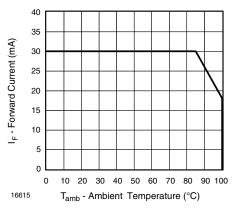
Figure 1. Forward Current vs. Ambient Temperature
