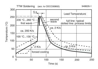
Figure 13. Double wave soldering of opto devices (all packages)
