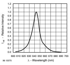
Figure 4. Relative Intensity vs. Wavelength
