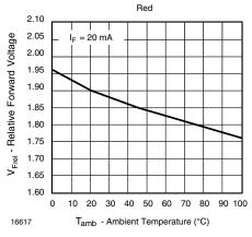
Figure 8. Forward Voltage vs. Ambient Temperature
