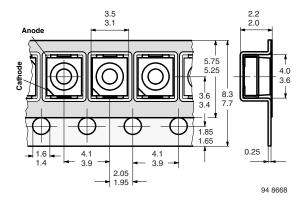
Figure 9. Tape dimensions in mm for PLCC-2
