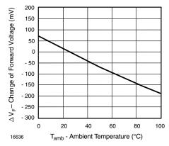
Figure 9. Change of Forward Voltage vs. Ambient Temperature
