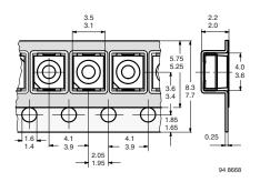
Figure 10. Tape dimensions in mm for PLCC-2
