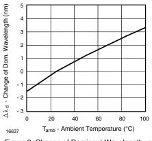
Figure 8. Change of Dominant Wavelength vs. Ambient Temperature
