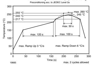
IR Reflow Soldering Profile for lead (Pb)-free soldering
