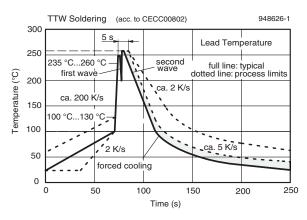
Figure 14. Double wave soldering of opto devices (all packages)
