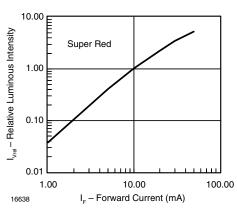
Figure 6. Relative Luminous Intensity vs. Forward Current
