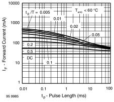
Figure 2. Forward Current vs. Pulse Length
