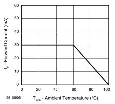
Figure 1. Forward Current vs. Ambient Temperature
