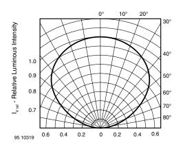
Figure 3. Rel. Luminous Intensity vs. Angular Displacement
