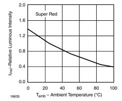
Figure 7. Rel. Luminous Intensity vs. Ambient Temperature
