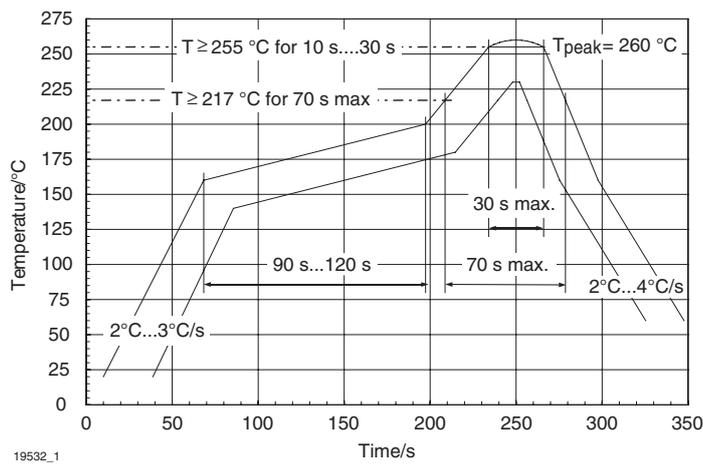
Figure 5. Solder Profile, RSS Recommendation
