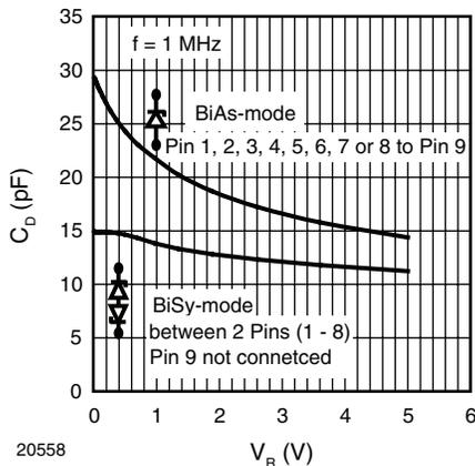
Figure 3. Typical Capacitance  $C_D$  vs. Reverse Voltage  $V_R$
