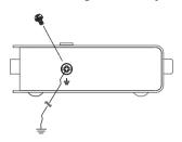
2. Make sure that the computer that the CE750L connects to and the monitor that the CE750R connects to are properly grounded.
