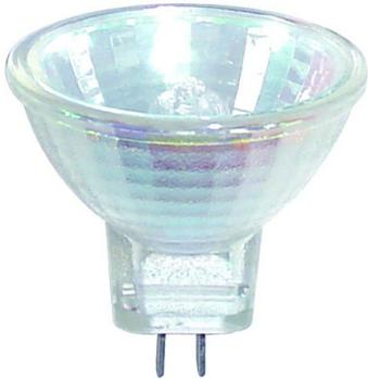
Multi faceted reflector (MR) halogen display low voltage lamps are ideal for down-lighting and accent lighting applications because of their small size, precise beam control, excellent white light and cool beam characteristics. Applications range from private offices, restaurants, retail displays as well as household. Beam patterns range from very narrow spot to wide floods.
