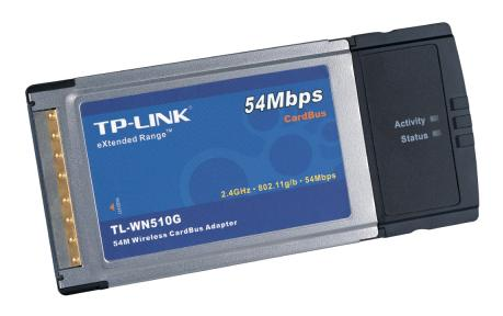
Wireless Roaming, can move among different AP with no break Adopts eXtended Range™ technology, 4-9 times the signal coverage of traditional 11b/g products
