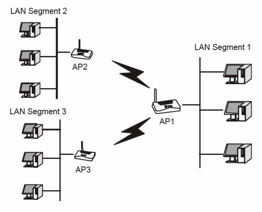
Figure 4-10 Point to Multi-point Bridge
