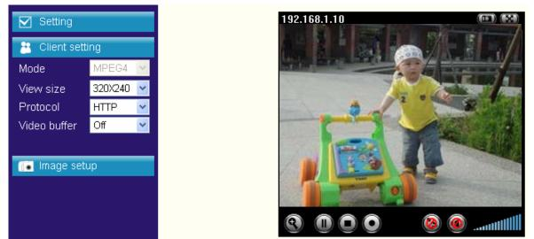
Click this button to configure the settings of IP Camera, which includes **Mode**, **View Size**, **Protocol**, and **Video Buffer**.
