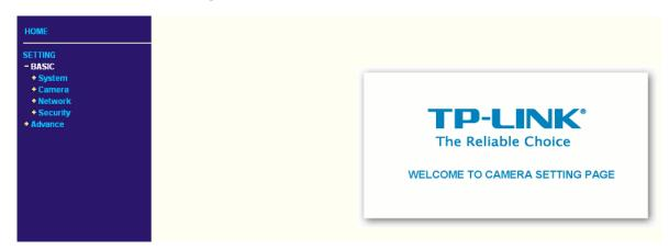
Click **BASIC** to display the submenus including **System**, **Camera**, **Network**, and **Security**.
