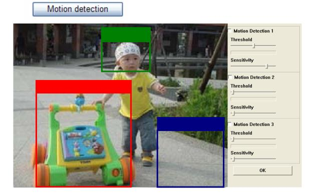
You can set motion detection on **motion detection page**. (Please go to "Setting  $\rightarrow$  Advance  $\rightarrow$  Motion detection  $\rightarrow$  Setting") For more details, you can check Section 6.5.
