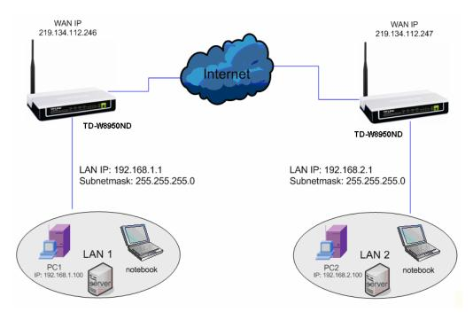
You could also use other VPN Routers to set VPN tunnels with TD-W8950ND. TD-W8950ND supports up to 10 VPN tunnels simultaneously.
