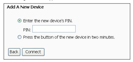
Step 2: Choose **Enter the new device's PIN** and enter the PIN code of the wireless adapter in the field behind PIN in the above figure. Then click Connect.
