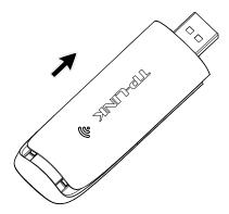
2. Insert the SIM card and the Micro SD card in the direction indicated on the Adapter.
