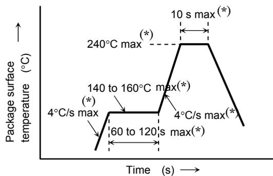
Temperature profile for Pb-free soldering (example)
