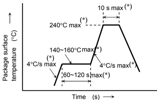
Temperature profile for Pb-free soldering (example)
