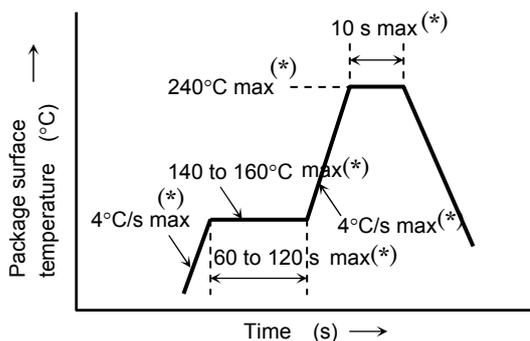
Temperature profile for Pb-free soldering (example)
