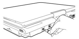
(Sample Illustration) Connecting the AC adaptor to the computer
