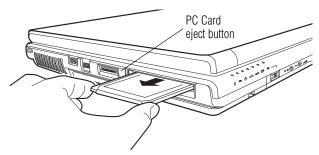
(Sample Illustration) Removing a PC Card
