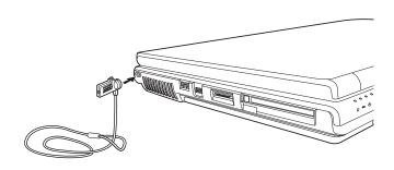
(Sample Illustration) Attaching security lock cable
