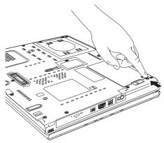
(Sample Illustration) Unlocking the battery release lock
