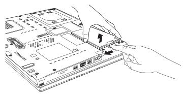
(Sample Illustration) Removing the battery
