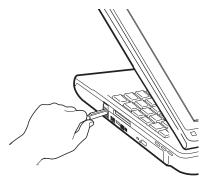
(Sample Illustration) Removing the Toshiba tablet pen from the slot on the tablet computer
