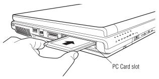
(Sample Illustration) Inserting a PC Card
