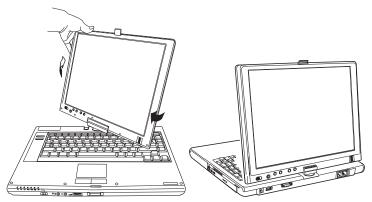
(Sample Illustration) Rotating the display panel clockwise 180°
