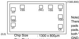
Chip Thickness: 280±20µm Chip Back : VDD level Pad Aperture : 88 x 88 µm Note) There are two VSS pads and two VDD pads. Please connect both VSS pads to GND, and connect both VDD pads to a power supply.
