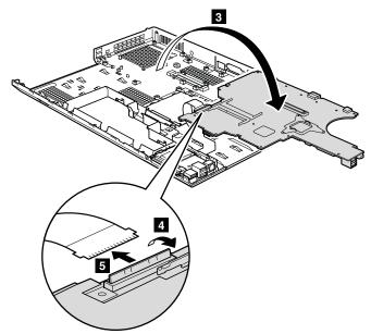
When installing: Make sure that the connector of the PC Card/Express Card slot assembly or PC Card/Smart Card slots assembly is attached to the system board firmly.
