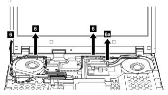
When installing: In ThinkPad W700ds, make sure that the cable connector 6a is attached firmly.
