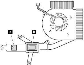
• Make sure that the fan connector is attached firmly.
