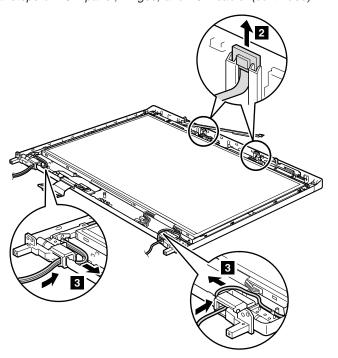
Table 43. Removal steps of LCD panel, hinges, and LCD cable (continued)
