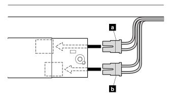
When installing: In some models, Make sure that connector that has pink cable and white cable a and the connector that has blue cable and white cable b are attached firmly.
