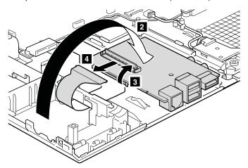
When installing: Make sure the connector is attached firmly.
