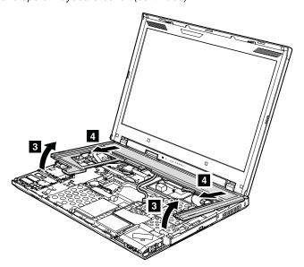
When installing: Make sure that all the claws are attached firmly.
