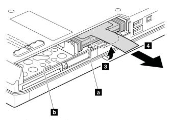
**When installing:** Make sure that the HDD connector or SSD connector is attached firmly.
