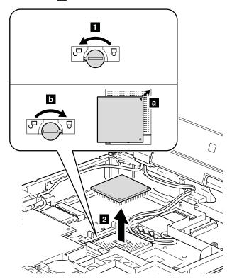
When installing: Place the CPU on the CPU socket **a**, and then rotate the head of the screw in the direction shown by arrow **b** to secure the CPU.
