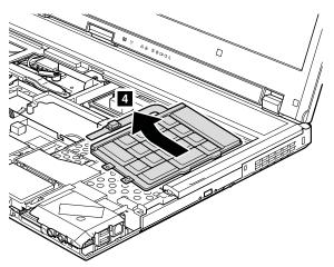
**When installing:** Make sure that the keypad edges **1** are under the frame as shown in this figure.
