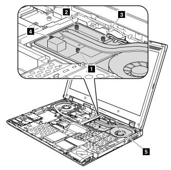
**Attention:** Do not handle the fan roughly. Improper handling of the fan can cause distortion or deformation and imperfect contact with components.
