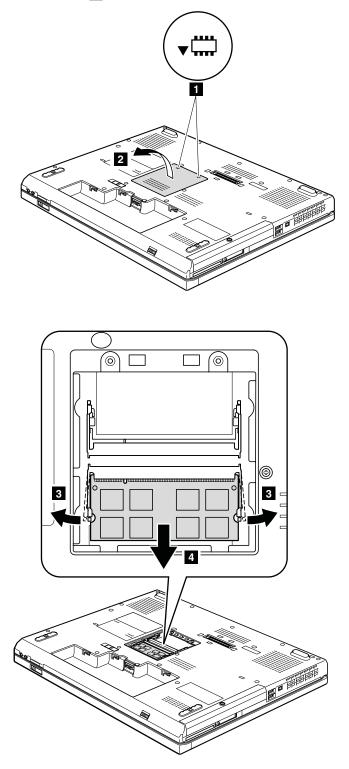
Table 15. Removal steps of DIMM slot cover and DIMM (continued)
