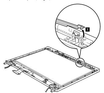
Table 43. Removal steps of LCD panel, hinges, and LCD cable (continued)
