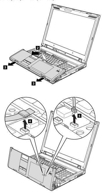
When installing: When you attach the palm rest, do as follows:
