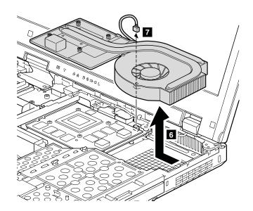
Table 30. Installation of the VGA thermal device/fan
