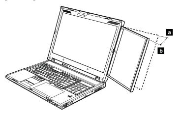
• To store the second screen in its slot, press the screen inside till it stops. Take your hand away and make sure that the screen is firmly locked in the slot. Unless you do this, the second screen might accidentally slide out.
