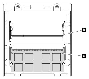
**When installing:** Insert the notched end of the DIMM into the socket. Press the DIMM firmly, and pivot it until it snaps into the place. Make sure that it is firmly fixed in the slot and does not move easily.
