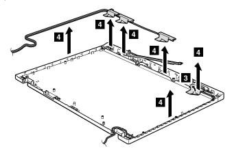
Cable routing: As you route the cables, make sure that they are not subjected to any tension. Tension could cause the cables to be damaged by the cable guides, or a wire to be broken. When attaching the antenna cable, route the cable as shown in this figure:
