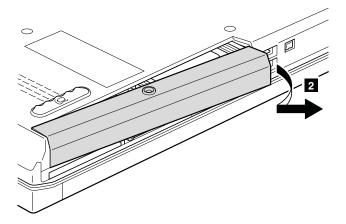
**Note:** Mounted number of the hard disk drive depends on the models. In models with RAID features, two hard disk drives that have same FRU no. must be used in slot 0 ( **a** ) and in slot 1 ( **b** ).
