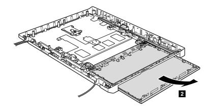
Table 48. Removal steps of second LCD hinges and second LCD rear cover (second LCD cover kit) (for ThinkPad W700ds) (continued)
