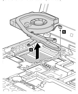
Table 28. Installation of the CPU thermal device/fan
