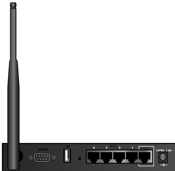
Figure 1-2: FWG114P Rear Panel
