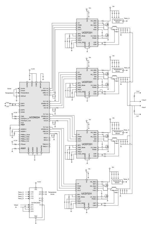
Figure 5. Typical Application Schematic Using UCD7231 Drivers
