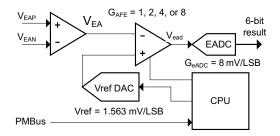
Figure 9. Analog Front End Block Diagram
