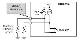
Figure 6. PMBus Address Detection Method
