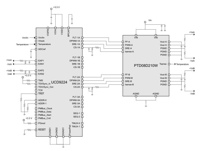
Figure 4. Typical Application Schematic Using PTD Driver Module
