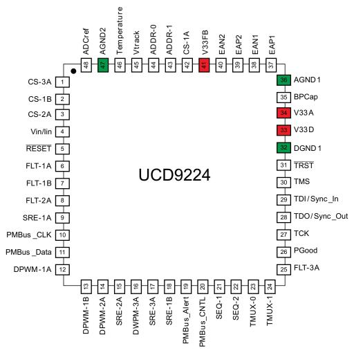
Figure 3. Pin Assignment Diagram
