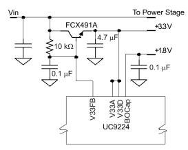
Figure 7. Series-Pass 3.3V Regulator Controller I/O
