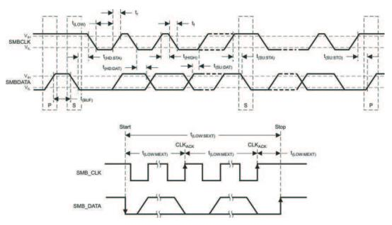
Figure 1. \l2C/SMBus/PMBus Timing in Extended Mode Diagram
