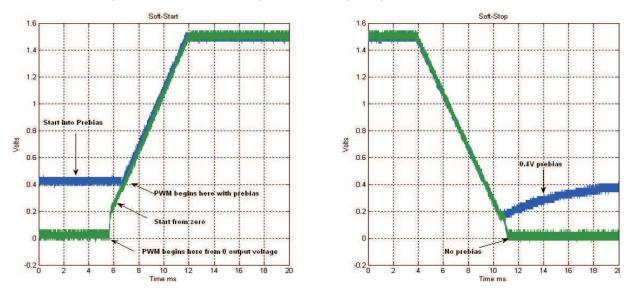
Figure 13. Start and Stop Ramps
