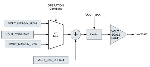
Figure 8. PMBus Voltage Adjustment Methods
