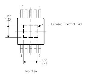
NOTE: All linear dimensions are in millimeters
