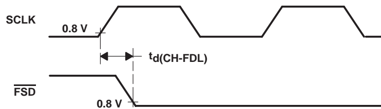
Figure 5–3. Master/Slave SCLK to \overline{\text{FSD}} Timing
