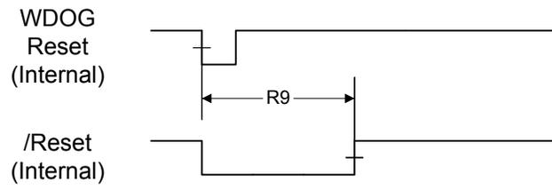
**Figure 17-13. LDO Reset Timing**
