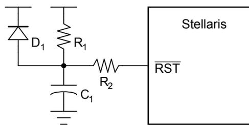
The  $R_1$  and  $C_1$  components define the power-on delay. The  $R_2$  resistor mitigates any leakage from the  $\overline{\text{RST}}$  input. The diode ( $D_1$ ) discharges  $C_1$  rapidly when the power supply is turned off.
