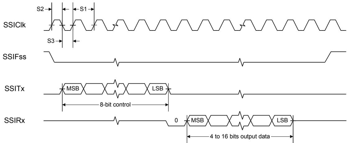
Figure 17-4. SSI Timing for SPI Frame Format (FRF=00), with SPH=1
