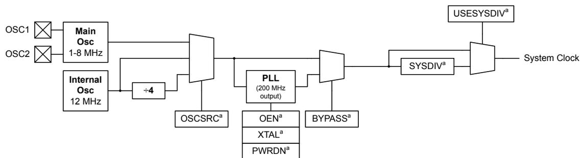
a. These are bit fields within the **Run-Mode Clock Configuration (RCC)** register.
