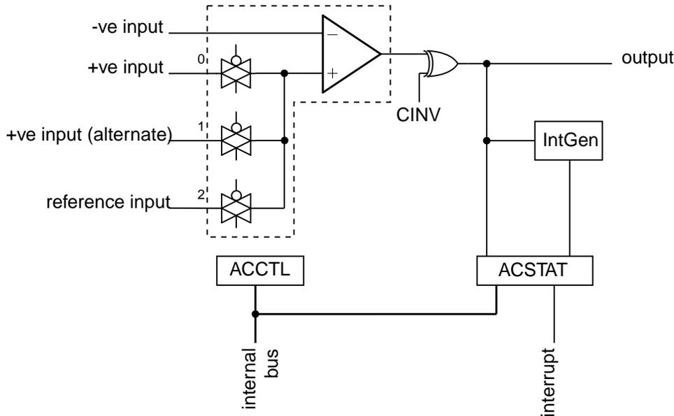
A comparator is configured through two status/control registers (**ACCTL** and **ACSTAT**). The internal reference is configured through one control register (**ACREFCTL**). Interrupt status and control is configured through three registers (**ACMIS**, **ACRIS**, and **ACINTEN**). The operating modes of the comparators are shown in the Comparator Operating Mode tables.
