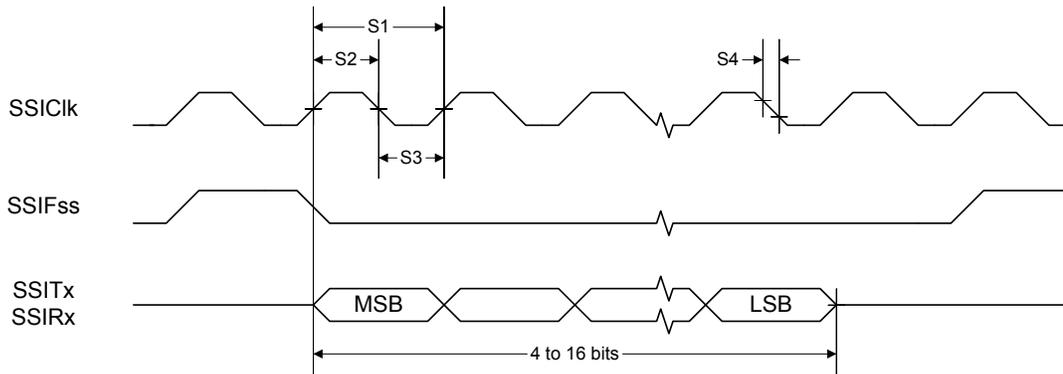
Figure 17-3. SSI Timing for MICROWIRE Frame Format (FRF=10), Single Transfer
