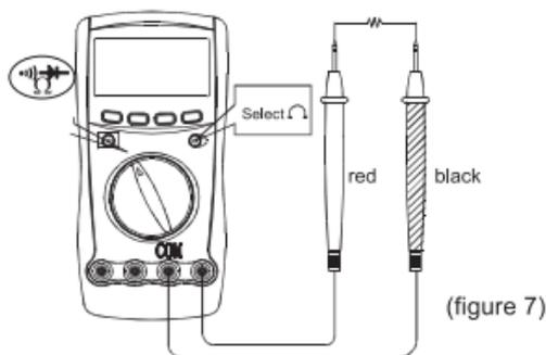
The resistance ranges are: 400.0Ω, 4.000kΩ, 40.00kΩ, 400.0kΩ, 4.000MΩ and 40.00MΩ. To measure resistance, connect the Meter as follows:
