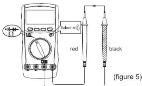
To test for continuity, connect the Meter as below:
