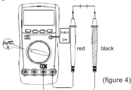
The DC Voltage ranges are: 400.0mV, 4.000V, 40.00V, 400.0V and 1000V. To measure DC voltage, connect the Meter as follows:
