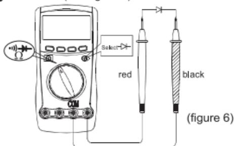
Use the diode test to check diodes, transistors, and other semiconductor devices. The diode test sends a current through the semiconductor junction, and then measures the voltage drop across the junction. A good silicon junction drops between 0.5V and 0.8V.
