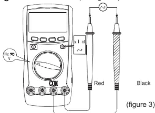
The AC voltage ranges are: 4.000V, 40.00V, 400.0V and 750.0V. To measure AC Voltage, connect the Meter as follows:
