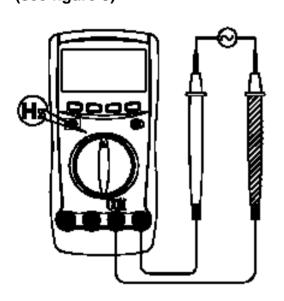
The measurement range is from 10Hz to 10MHz. To measure frequency, connect the Meter as follows:
