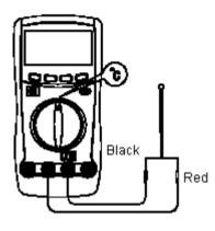
The temperature measurement range is -40°C to 100°C to measure temperature, connect the Meter as follows:
