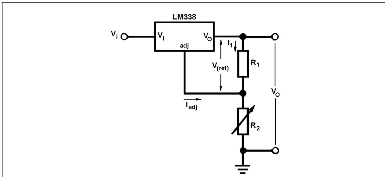
Since the 50 $\mu$ A current from the adjustment terminal represents an error term, the LM338 was designed to minimize  $I_{adj}$  and make it very constant with line and load changes. To do this, all quiescent operating current is returned to the output establishing a minimum load current requirement. If there is insufficient load on the output, the output will rise.
