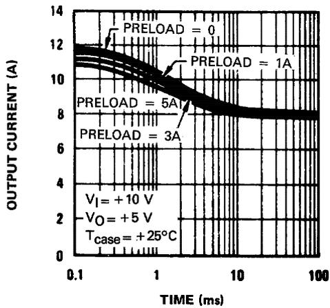
Figure 6 : Adjustment Current
