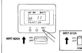
The example shows TV channel display on the WRT-810A(68) or WRT-820A(68).
