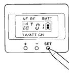
The current input attenuation setting in decibels will appear on the display.  Switching from channel set mode to attenuation display/set mode
