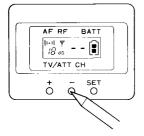
If you keep either button pressed, the input attenuation setting will be incremented or decremented successively until it reaches 0 or 21 dB.
