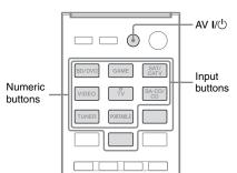
1 While holding down the input button of which you want to change the assignment, hold down AV I/<sup>(1)</sup>.
