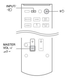
1 While holding down MASTER VOL –/ ∠ –, press I/ () and INPUT/-€.
