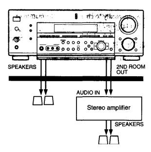
You can select the analog audio signals for output to a stereo amplifier or speakers in another room. For details on the connection, see pages 14 and 18.
