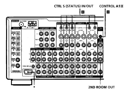
\* This jack is intended only for use in the manufacturing and servicing of the unit.
