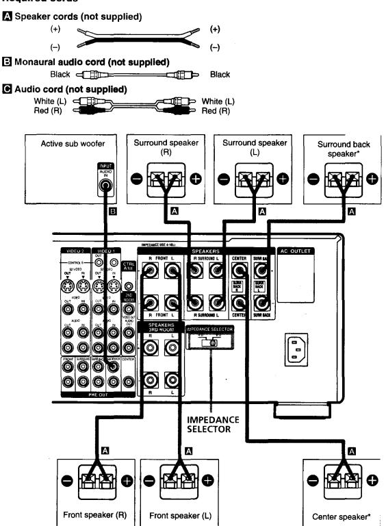
You can use the connected center and surround back speakers as surround back right and left speakers. (See "Setting to the 7.1 channel mode" on page 28.) Make sure to connect correctly as indicated on the rear panel.
