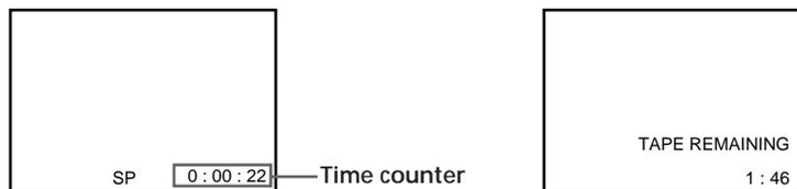
To check the remaining time of a T-140, T-180 or longer tape, set TAPE SELECT in the ADVANCED OPTIONS menu to "180." (For details, see page 58.)
