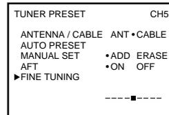
**4** Press CURSOR ←/→ to adjust to a clearer picture, then press EXECUTE. Note that the AFT setting switches to OFF.
