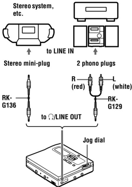
When connecting a line cable to the  $\odot$ /LINE OUT jack of the recorder, be sure to set the “AUDIO OUT” parameter for the  $\odot$ /LINE OUT jack.
