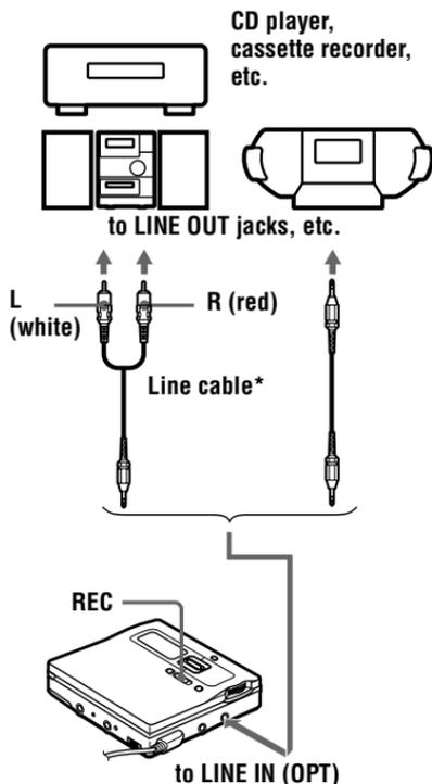
\* Use the connecting cords without an attenuator. To connect to a portable CD player having a stereo mini-jack, use the RK-G136 connecting cord. For more information on connecting cords, see "Optional accessories" (page 93).
