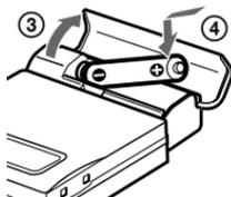
Insert a LR6 (SG) alkaline dry battery.
