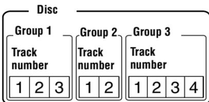
It is convenient for managing multiple CD albums recorded in MDLP (LP2 stereo/LP4 stereo) mode onto a single MD. You can create a maximum of 99 groups on a disc.
