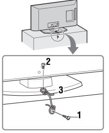
Install a wood screw (4 mm in diameter, not supplied) in the TV stand.
