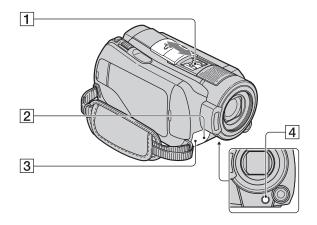
■ Active Interface Shoe j Attemptson The Active Interface Shoe supplies power to optional accessories such as a video light, a flash, or a microphone. The accessory can be turned on or off as you operate the POWER switch on your camcorder. Refer to the operating instructions supplied with your accessory for details.
