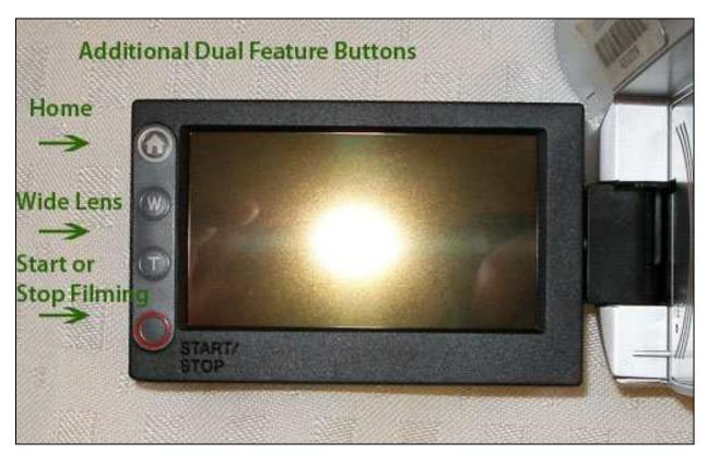
**Step 7:** Use the buttons on the LCD screen or camera to film, and start and stop.
