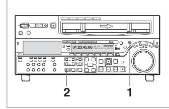
Press the RECORDER button, turning it on.
