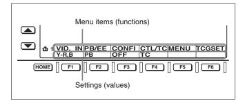
In the figure above, Y-R,B (analog component signals) is selected as the setting for VID.IN, the menu item for button F1. This manual refers to this as "F1 (VID.IN) in function menu HOME page is set to Y-R,B."
