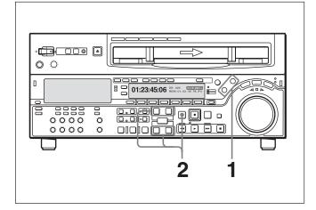
**1** Press the RECORDER button or PLAYER button to select the VTR on which you wish to operate.
