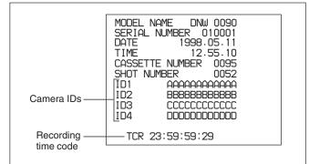
The details in the shot data depend on the shooting conditions. If because of the devices used there is no shot data on a part of the tape, it appears as blank.
