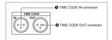
**1 TIME CODE IN connector (XLR 3-pin, female)** To record time code from an external device, input a time code signal from the time code output connector of the other device.
