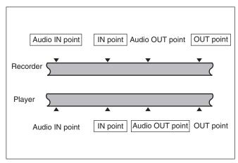
You can set audio cut in, crossfade, fade in, and fade out effects, including their durations, by menu selection. For details, refer to the Installation Manual.
