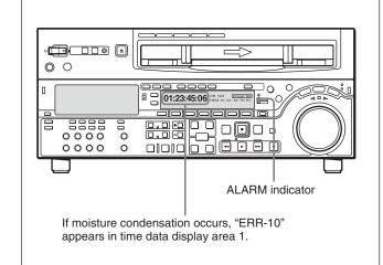
If this happens, the drum and capstan motors stop and the cassette is automatically ejected. Then, the durm starts to rotate again to dry its surface. In this state, the unit is not operable. When the moisture has evaporated, the error message disappears and the ALARM indicator goes off.
