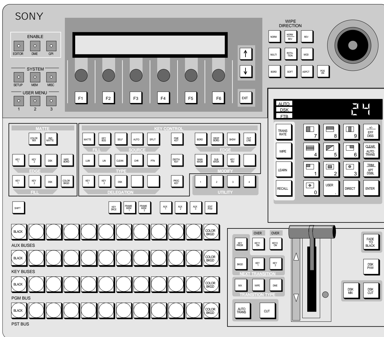
BKDS-2010 Control Panel Top View
