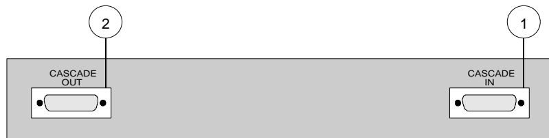
BKDS-8061 Shot Box Control Unit Rear View
