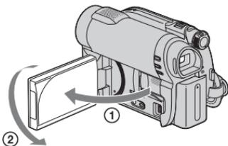
Open the LCD panel 90 degrees to the camcorder (①), then rotate it 180 degrees to the lens side (②).
