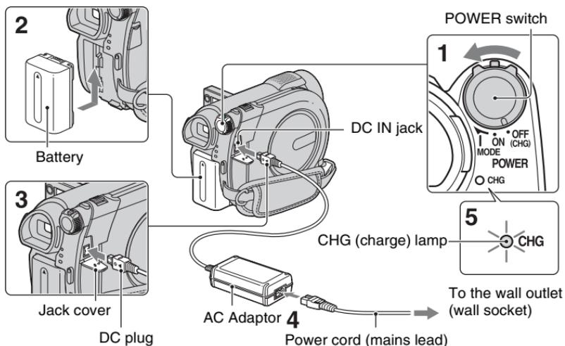
You can charge the “InfoLITHIUM” battery pack (H series) (p. 121) after attaching it to your camcorder.
