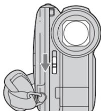
After recording, set the LENS COVER switch to CLOSE to close the lens cover.
