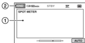
① Touch the point where you want to fix and adjust the exposure on the screen.
