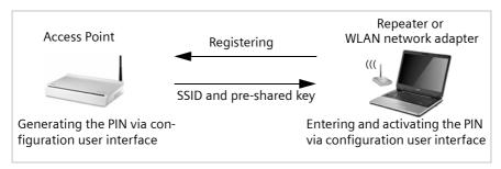
WLAN adapters without WPS can also be set up manually, i.e. the SSID and key must be entered manually. How you can find out which SSID and which pre-shared key is set, you can read in chapter "Configuring wireless connections" on page 87.
