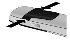
> Place the handset in the base/charger with its display facing forward.
