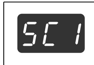
The display will show the number of the [SCAN MENU] key that you pressed, and the number will light and the SCAN indicator will be blinking.
