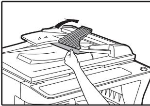
**2** Open and close the SPF/RSPF to make the misfeed location indicator stop blinking.
