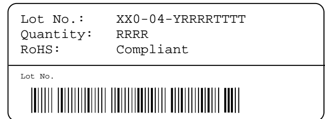
Figure 14: First label on reel: XX = Sensor Type (71 for SHT71), 04 = Chip Version (V4), Y = last digit of year, RRRR = number of sensors on reel, TTTT = Traceability Code.
