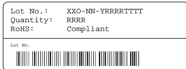
Figure 18: First label on reel: XX = Sensor Type (21 for SHT21), O = Output mode (D = Digital, P = PWM, S = SDM), NN = Chip Version, Y = last digit of year, RRRR = number of sensors on reel, TTTT = Traceability Code.
