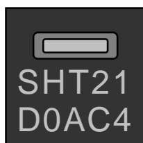
Figure 17 Laser marking on SHT21. For details see text.
