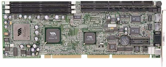
The **SBC81610** CPU card is an industrial grade CPU card incorporating the VIA VT8601T chipset and the VT82C686B with built-in AGP-2x VGA controller, both ensuring its compatibility with PCI bus passive backplanes. Its 4-layer structure reduces signal noise and built-in power management feature. These advanced concepts along with the PCI Local Bus architecture bring outstanding performance to Windows-based applications.
