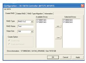
\* The Create Option is active for RAID 1, 5 and RAID 0+1 only. The 'Create Only' option will destroy data in both of the selected drives. The 'Dupli cate/Rebuild' option will keep the source drive data and copy source drive data into the target drive.
