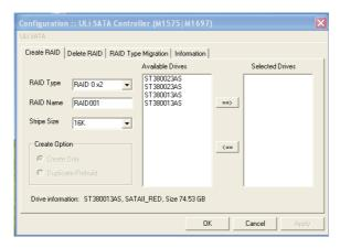
Click the desired drive from the 'Available Drives' list, use the right arrow key to move the drives that you plan to use to the 'Selected Drives' list. You can select array type from the 'RAID Type' pulldown menu and select stripe size for RAID 0 from the 'Stripe Size' pull-down menu.
